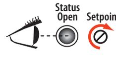
3. Turn the setpoint screw an additional 1/4 turn clockwise for operational margin.
