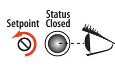
3. Turn the screw an additional 1/4 turn counter-clockwise for operational margin.
