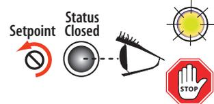
2. Slowly turn the setpoint screw clockwise until the Status OPEN LED just turns ON.
