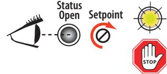
2. Slowly turn the screw counter-clockwise until the Status CLOSED LED just turns ON.
