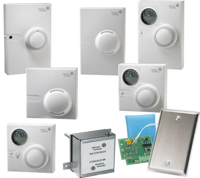
The NS Series Network Zone Sensors are designed to function directly with the *Metasys* system family of FEC field controllers. Several models of network zone sensors monitor room temperature. Options are available to also monitor zone humidity, carbon dioxide (CO<sub>2</sub>), local temperature setpoint adjustments, and other variables. This data is transmitted to a field controller on the SA Bus.
