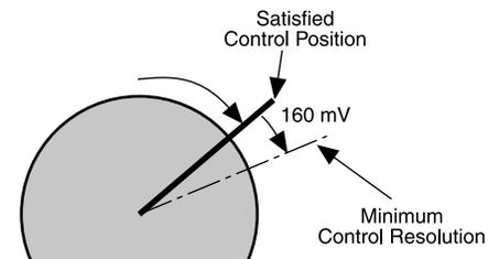
**LF Actuator responds to a 200 mV signal when reversing direction from stop position.**
